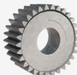
Near net pinions Press forging Diameter up to 180 mm Thickness between 50 and 90 mm Gear module \geq 6
